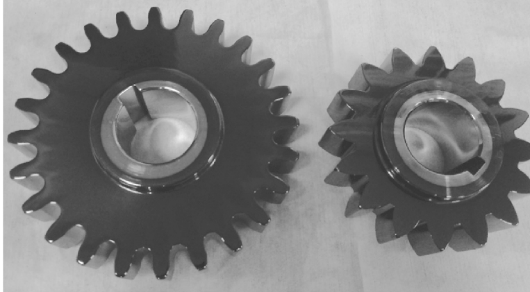
Figure 17.16 Gears with diamond-like carbon film deposited on the surface.
