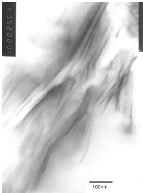
Fig. 14 TEM micrograph of POBDS–VMT nanocomposite (Reproduced with permission from Ref. [202])
